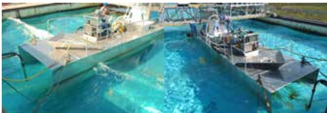
Figure 4. Gravity skimmer 12 m prototype testing at Ohmsett.
