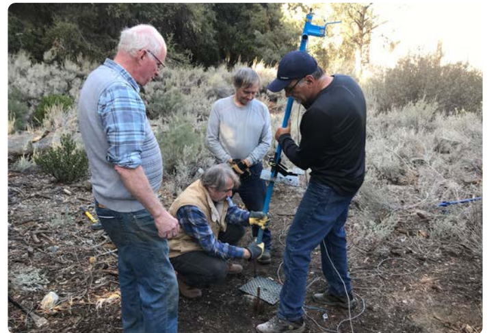
Using seismic equipment in hard-rock mountain terrain of California.
